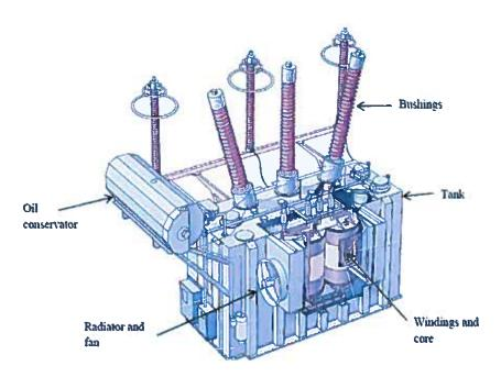
The core is made of silicon steel and is laminated with an inorganic coating. The silicon steel is layered in pieces and shaped into the legs and yokes of the core. Cores typically consist of two, three, four or five legs depending on the number of phases, capacity and transport restrictions.
